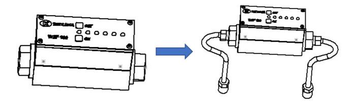
6.3. Attach the indicator with the tubes to the filter with the screwed reducers. Remember that the direction of flow on the indicator and filter should be the same.
