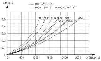
\* Reference diagram for models with filtering element = 25  $\mu m$
