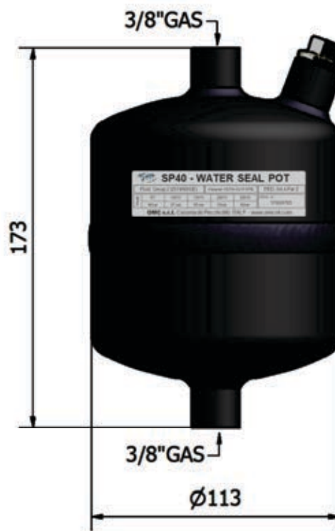
SP40 Available on request WATER SEAL POT FOR USE ON STEAM PN40 - ASTM A216 WPB Material
