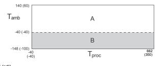
$T_{amb}$  = Ambient temperature °F (°C)  $T_{proc}$  = Process temperature °F (°C) A = All available electronic options
