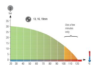
MAXIMUM WORKING PRESSURE 15 BAR AT 100°C
